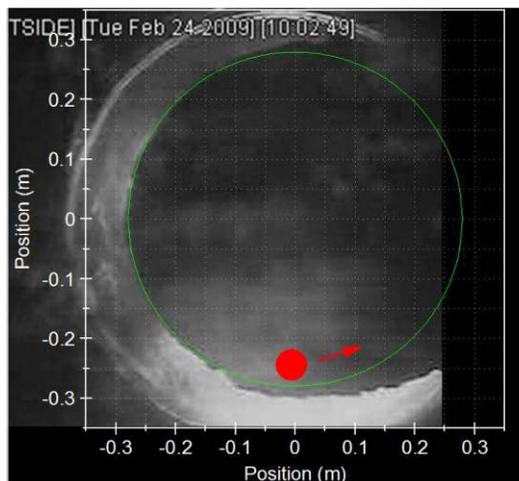
Figure 4. Determined arc position superimposed on top of a video frame at an instant. The arrow indicates the direction of arc motion, as observed in both the video and the arc position data.
