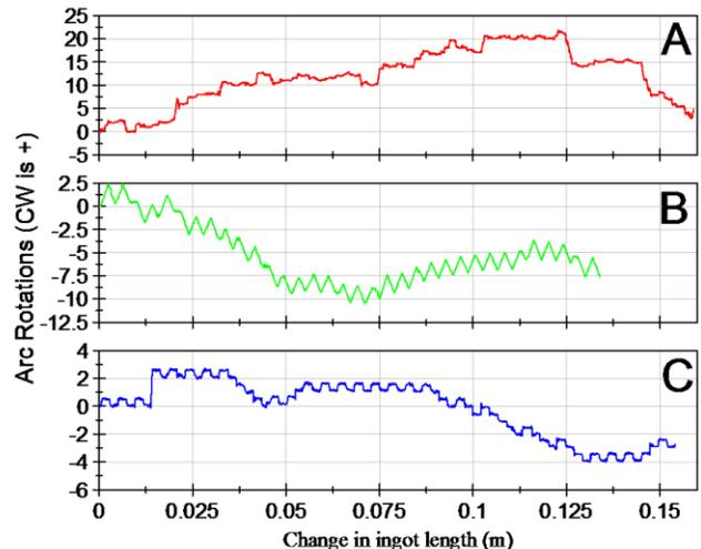
Figure 8. Arc rotation about the axis of the furnace when viewed from above where 1 rotation is  $2\pi$  radians. The letters correspond to those in Fig. 7.
