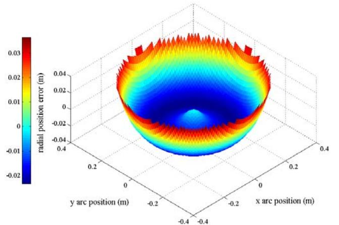
Figure 3. The radial position difference (error) between FEM arc locations and calculated arc locations using the single arc method.
