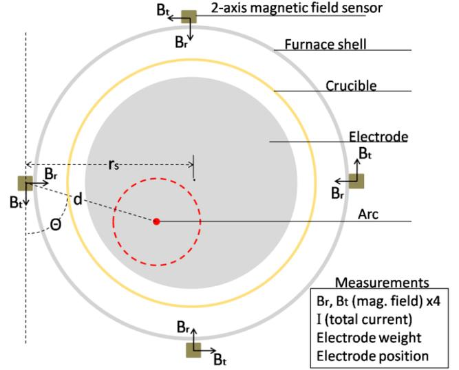
Figure 2. Overhead view of the experimental set-up. The red dotted line is to show that the found arc location with the single arc method could actually be a locally axisymmetric region of arcs (center of the arcs).
