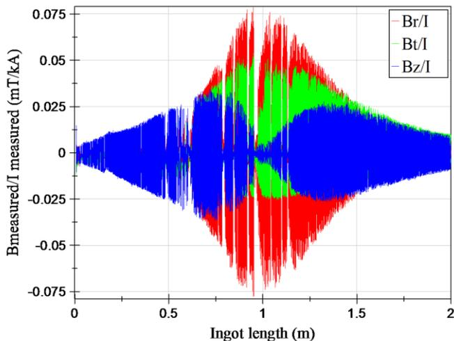
Figure 5. Waveform showing some of the measurements during a melt. The sensor was located at a position corresponding to an ingot length of about 1m.
