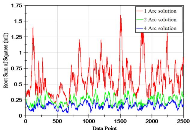
Figure 6. The RSS for the difference between the measured magnetic fields and the calculated magnetic fields for the best found arc positions when solving for the indicated number of arcs.
