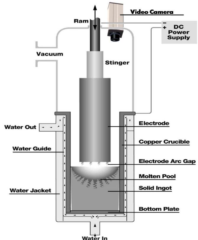
Figure 1. Cross Section of a typical industrial VAR furnace. Sketch is courtesy of ATI-Allvac, with a modification to show the video camera's location during the experiments.
