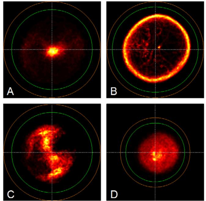
Figure 7. Four types of arc distribution patterns observed during Ti. VAR melting. Color intensity (hot color map) corresponds to the number of instances the center of the arcs were found at the corresponding position. The inner circle represents the electrode and the outer circle the crucible. The view is looking down the axis of the furnace.
