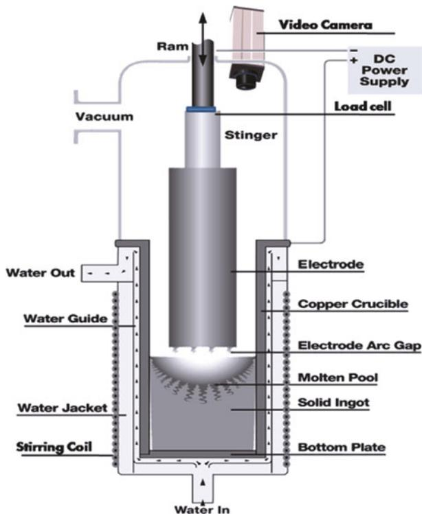
Fig. 1—Cross section of the VAR furnace. Sketch is courtesy of ATI Allvac, with a modification to show instrumentation.
