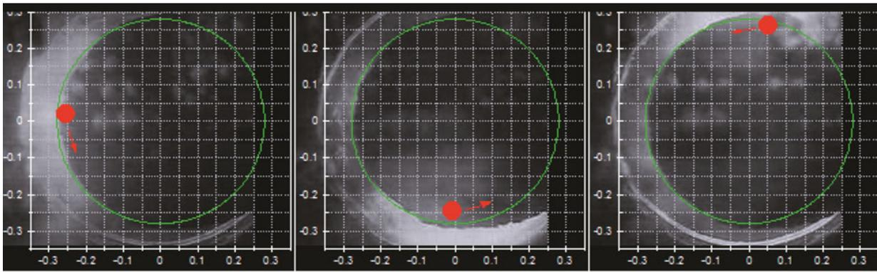
Fig. 6—Determined arc position superimposed on top of three video frames spanning a period of less than 20 s. The arrow indicates the direction of arc motion as observed in both the video and the arc position data.
