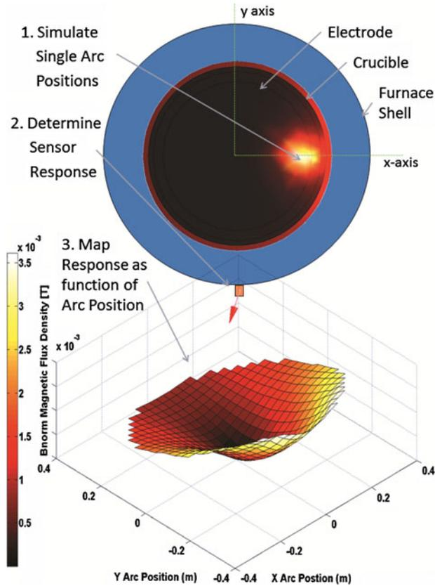
Fig. 2—At the top is an overhead view of the current density just below the ingot surface as determined by the FEA for a single-arc simulation. At the bottom is the magnitude of the normalized magnetic flux density vector for a sensor located at an  $x$ - $y$  coordinate of  $(0, -0.64)$  as a function of the position of a 35-kA arc center.
