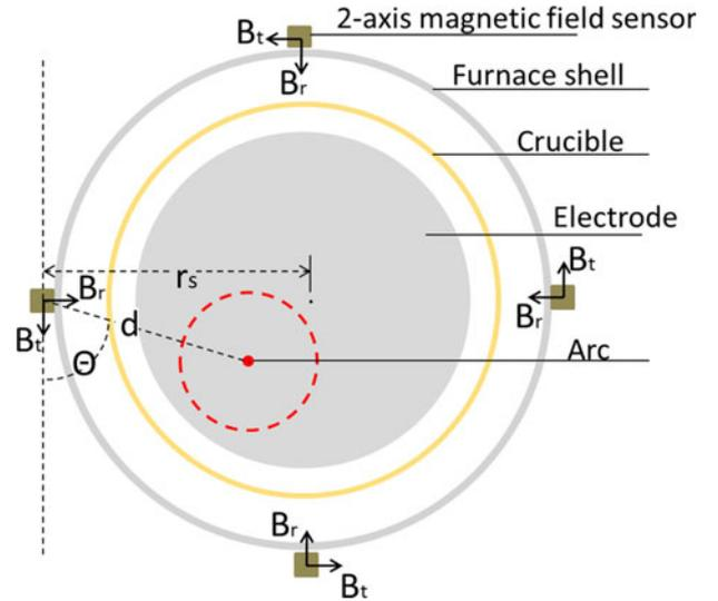
Fig. 3—Diagram of the setup for arc position determination. Determination is insensitive to the arc diameter, as indicated by the dotted line.
