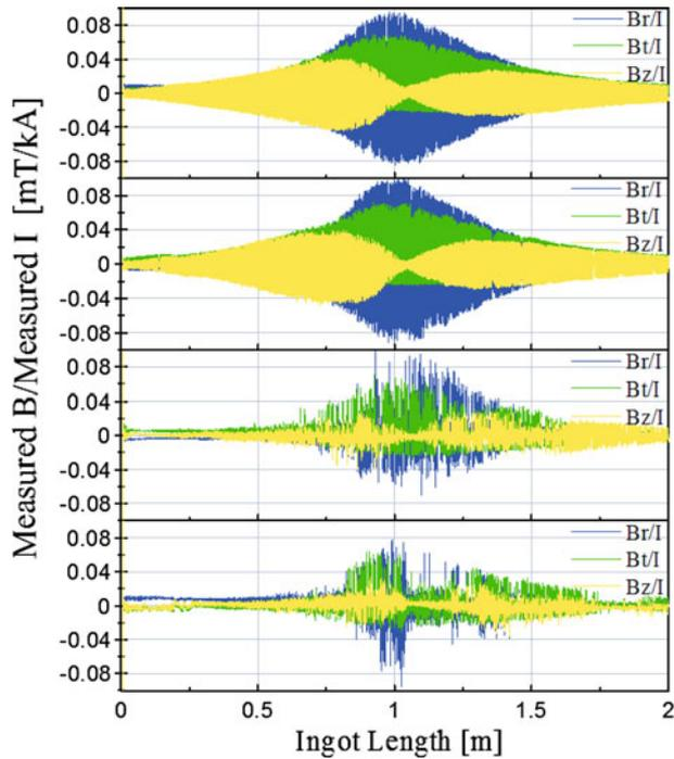
Fig. 5—Waveforms of experimental results showing the signal due to arc movement during four final Ti-6Al-4V VAR heats. The magnetic sensor was located at a position corresponding to an ingot length of about 1 m. The VAR process parameters were the same for each.
