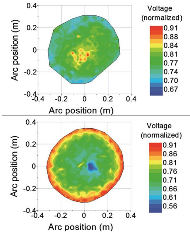
Fig. 8—Relation of furnace voltage to arc position. At top is the relation typically seen for heats dominated by a centered arc distribution, and at bottom is a correlation typical for heats dominated by a ring distribution.
