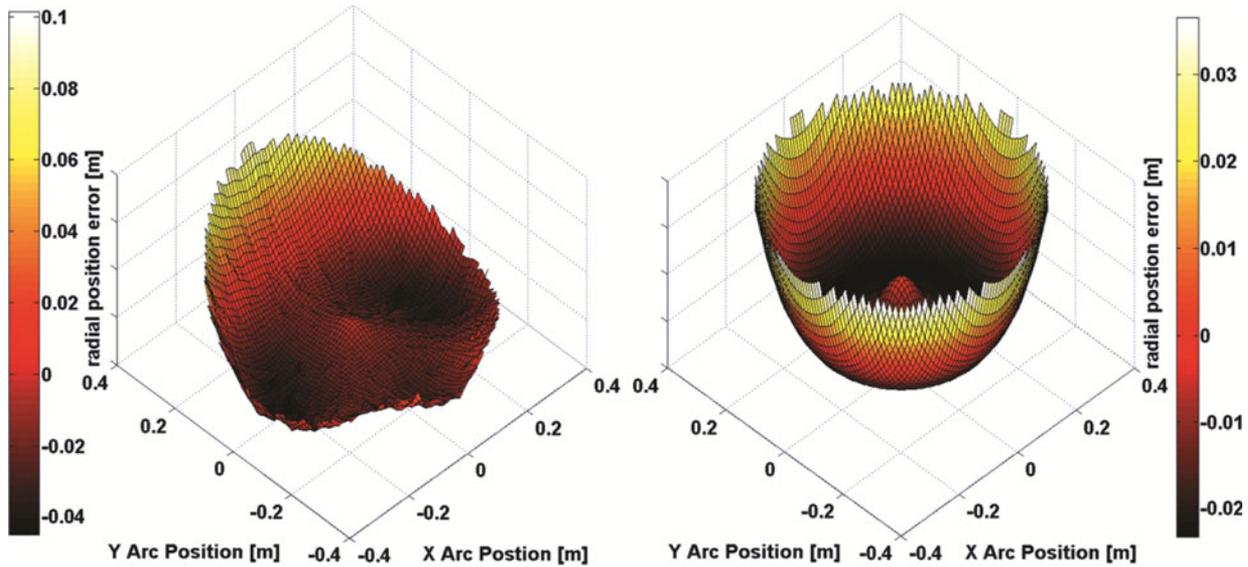
Fig. 4—The radial position difference (error) between FEM arc locations and calculated arc locations using the single arc method. At the left is the error for a single sensor located at (0, -0.64). At the right is the error when averaging the position data from the four sensors.
