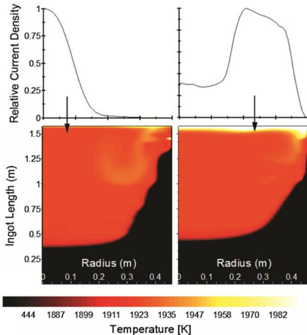
Fig. 9—The temperature profile in the liquid and mushy zones for two cases of VAR melting of Ti-6Al-4V. The case on the left is for the predicted current density into the ingot for the center arc-distribution mode, and the case on the right is for the ring distribution mode. The distribution was considered axisymmetric and constant over the duration of the melt.
