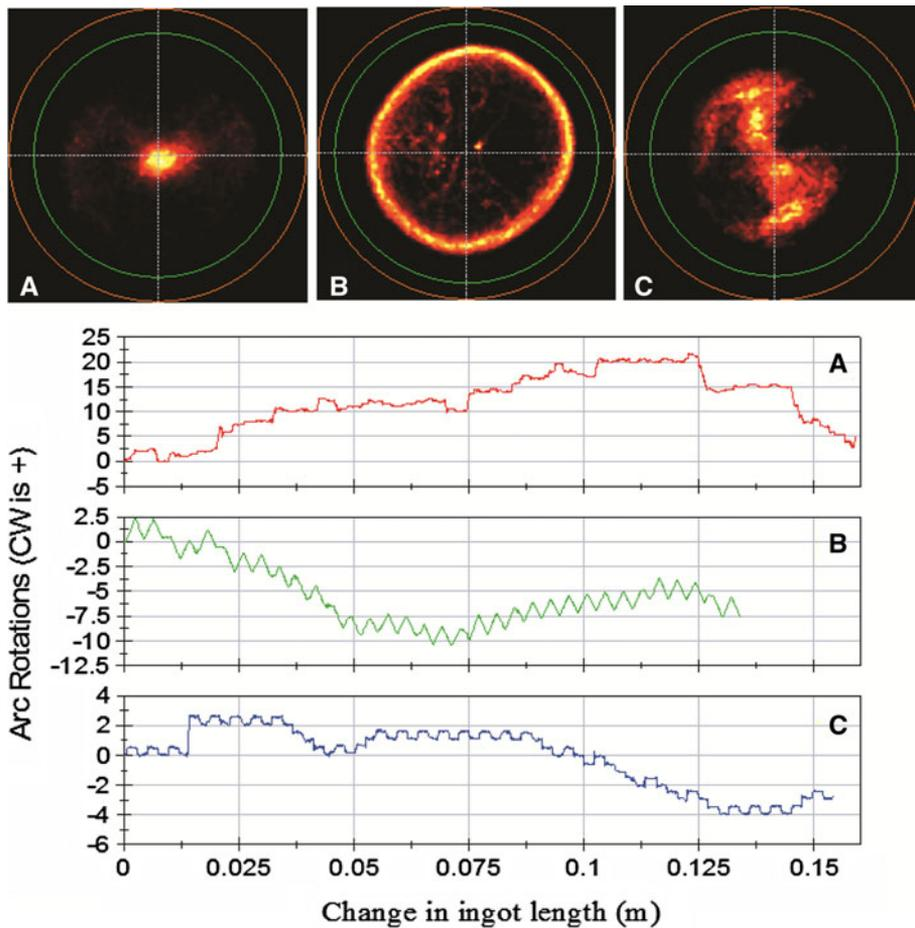
Fig. 7—Three types of arc distribution and motion observed during final Ti-6Al-4V VAR. Distribution is shown by color intensity (hot color map) corresponding to the number of insistences the arc center was found at the corresponding position. The inner circle represents the electrode and the outer circle the crucible. Azimuthal arc motion is shown in terms of arc rotations where one rotation is  $2\pi$  radians. The view is looking down the axis of the furnace.
