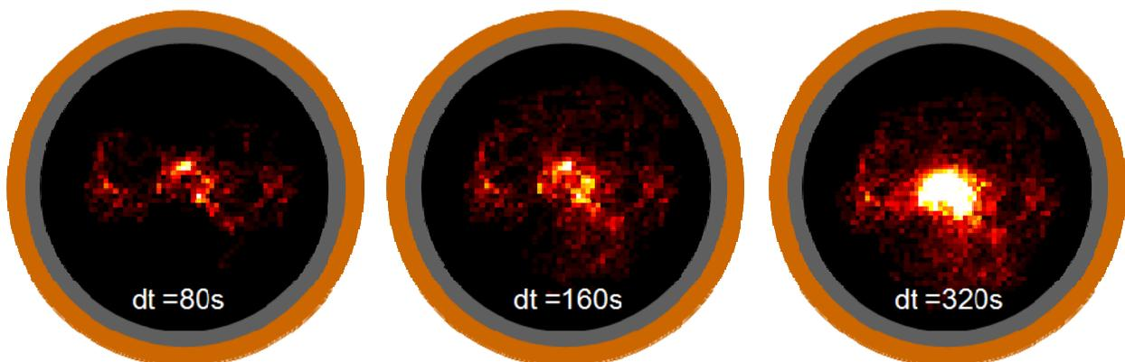
Figure 3 : Overhead view of the predicted arc distribution in the VAR furnace over increasingly long time scales. Color intensity corresponds to the number of arc location predictions in each location bin. The dark circle is the electrode.
