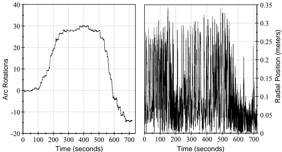
Figure 2: Arc rotations about the center of the furnace axis when viewed from above (left) and radial position (right) of the average predicted arc location. One arc rotation is  $2\pi$  radians, and the positive direction is clockwise.
