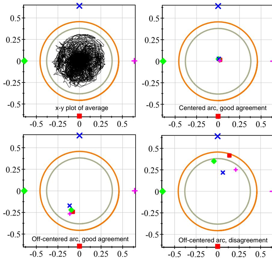
Figure 1 : The average of the predicted arc locations over 720 seconds of melt time (top-left) and a comparison of arc location predictions from the individual sensors at 3 instances; The dimensions are in meters, and the markers represent actual sensor location in addition to the location prediction. The outer circle is the crucible, and the inner circle is the electrode.
